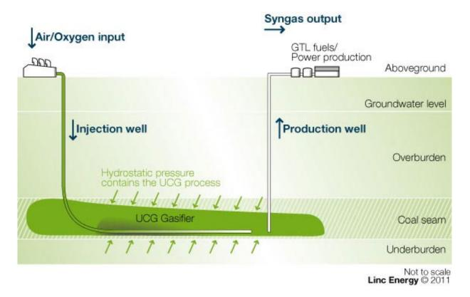
The key breakthrough in Linc Energy's UCG technology has been the use of horizontal directional drilling, similar to what is used to hydrofrack shale. Traditional UCG used simple vertical wells and it was always a steep challenge to both control the combustion and to maintain communication between the two wells for the effective flow of gas. By using directional horizontal drilling Linc can establish clear flow through between the two wells. Linc has also developed proprietary ignition,
