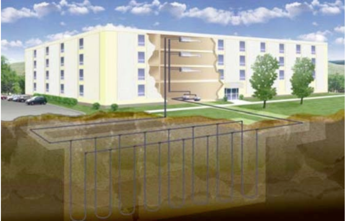
Figure 1-5. Diagram of Vertical Loop System source: McQuay International, 2009.
