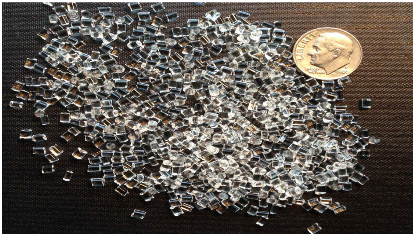
Novomer thermoplastic pellets are 40% CO 2 by weight.
