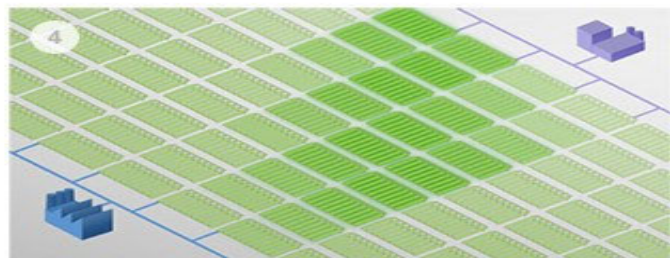
4 The process occurs continuously for up to 8 weeks before the capsules are flushed and reinoculated on a staggered basis.
